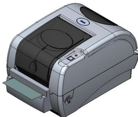
Fig. 28 Complete label installation in cutter mode
