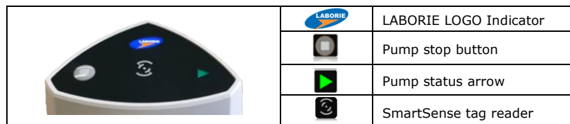
Figure 78: Status of the Pump
