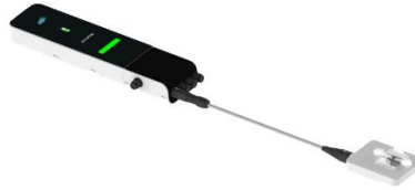
Figure 11: Roam NXT, PIM NXT for Fluid, and Pressure Transducer Connected
