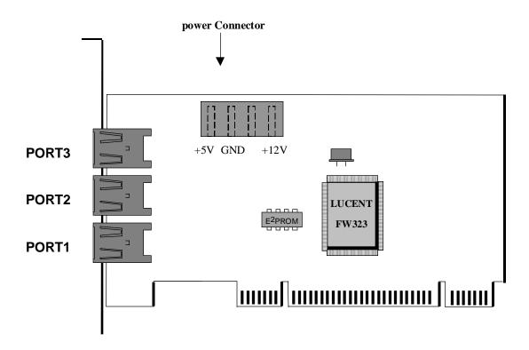
**Power Connector**: You can optionally conncet the power connector to the power supply if necessary.
