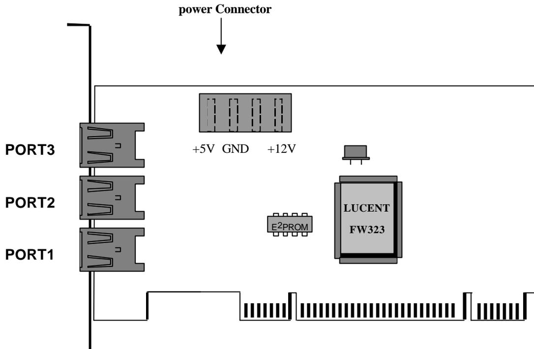
**Power Connector:** You can optionally connect the power connector to the power supply if necessary.
