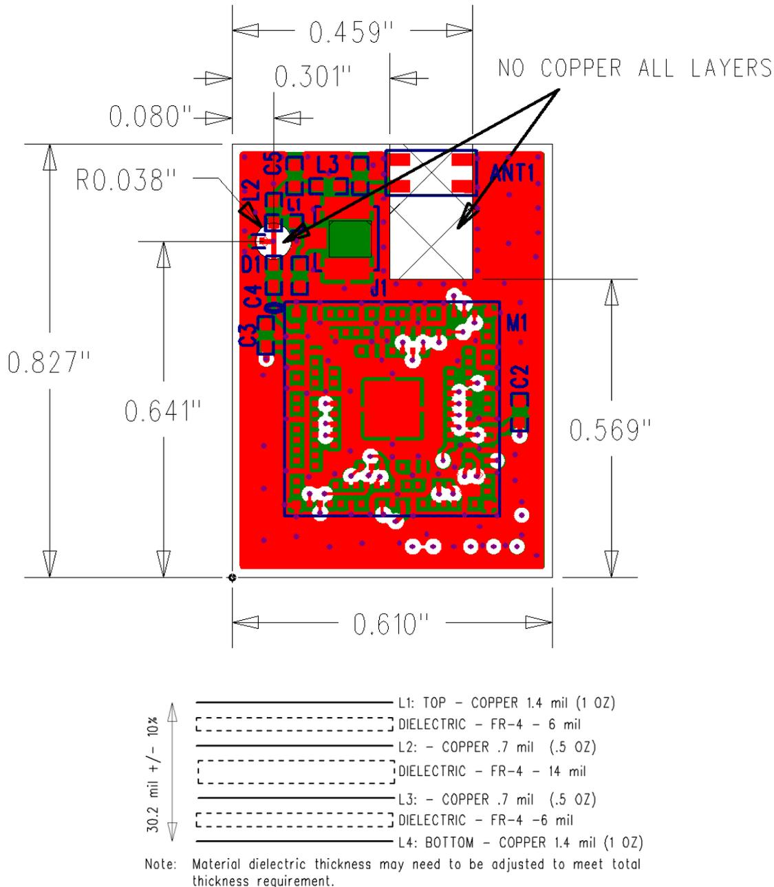
**Figure 1 SIP Module with Chip Antenna Reference Design**
