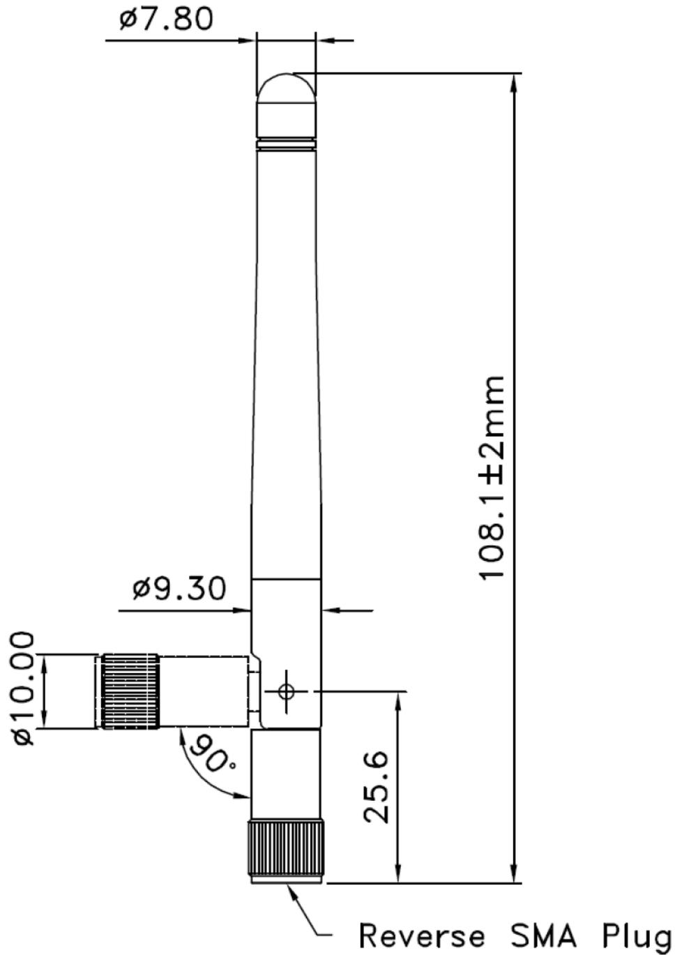
Figure 11 LSR 2.4 GHz Dipole Antenna Dimensions
