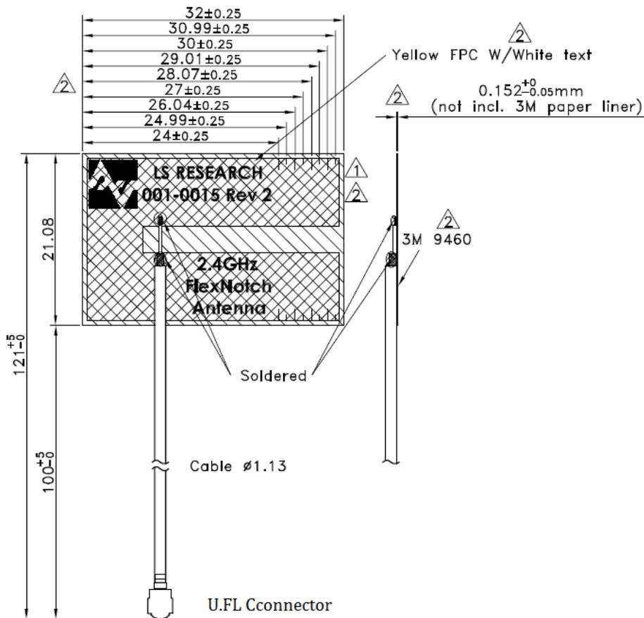
**Figure 10 LSR 2.4 GHz FlexNotch Antenna Dimensions**
