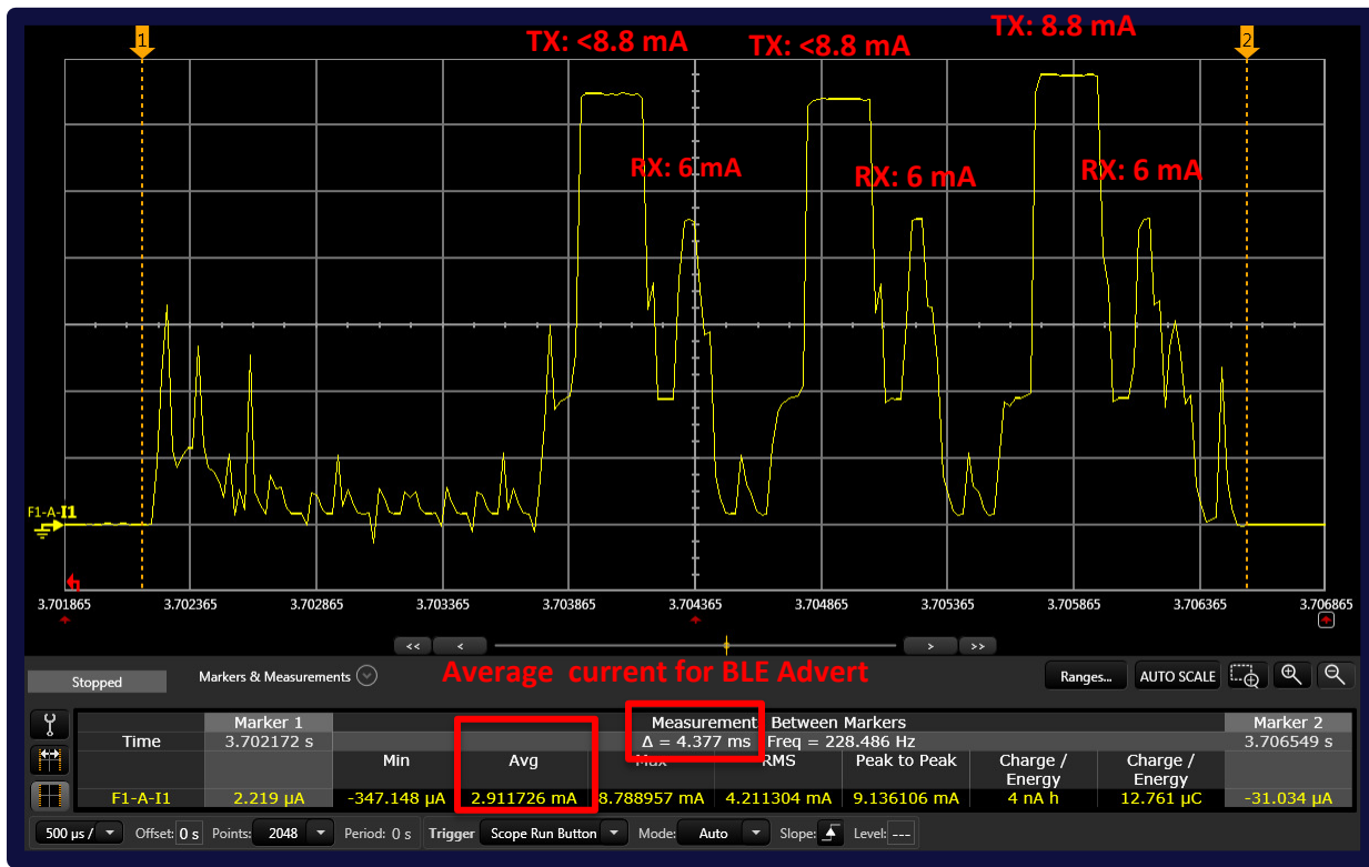
Figure 4: Typical peak current consumption profile (with DCDC ON) during advertising in slave mode @ TX PWR +4 dBm. UART is OFF
