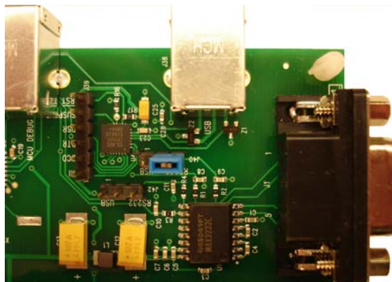
Figure 3-5. Jumper Set For RS-232 Serial Communications
