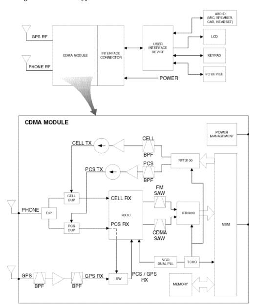
The Module card includes the following circuits, with the necessary filtering and AGC circuits to meet performance requirements.
