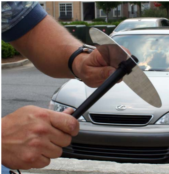
Figure 4 - 8. Putting ground plane on antennas
