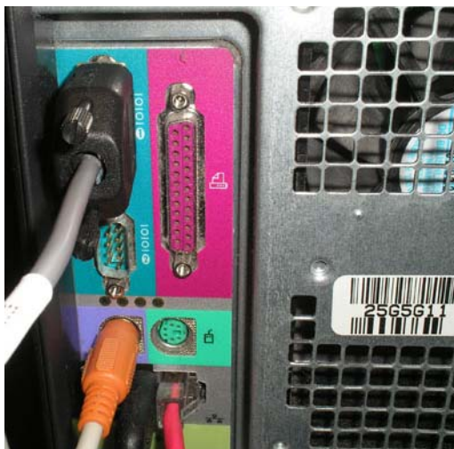
Figure 3 - 2. Serial cable plugged into COM 1
