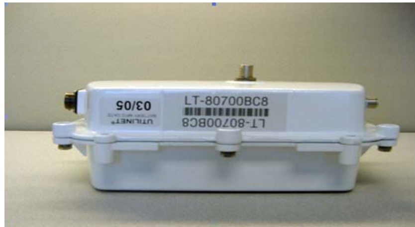
Figure 5 - 5. New battery date label affixed to concentrator enclosure
