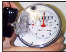
Figure 2.4 Applying moisture compound
