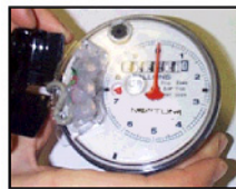
Figure 2.4 Applying moisture compound
