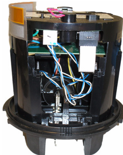
Figure 2.1 Serial connection between module and meter
