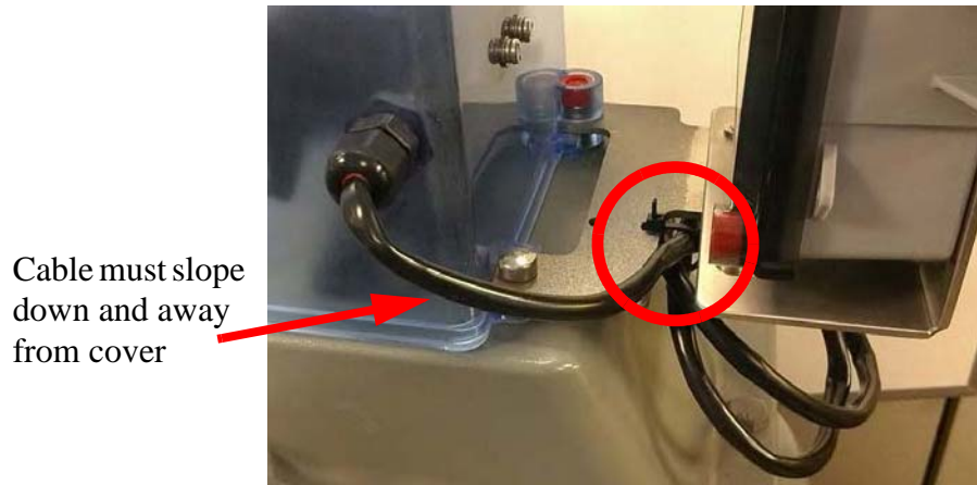
Figure 5 - 18. Route and Attach the Excess Cable
