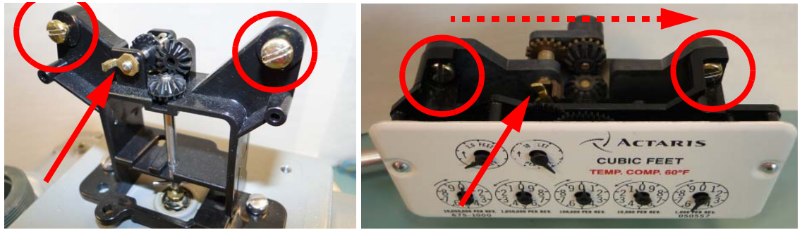
Figure 5 - 8. Index Screw and Drive Details
