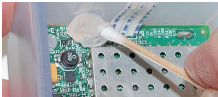
Figure 8 - 23. Force the Compound Between Connector Pins
