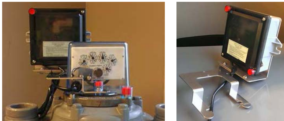
Figure 3 - 30. GPR at Left Rear - Using 28-1443 Bracket
