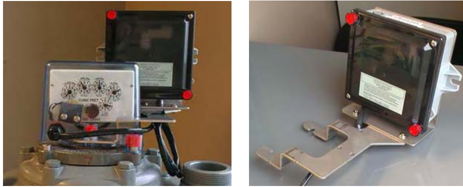
Figure 3 - 31. GPR at Right Rear - Using 28-1440 Bracket
