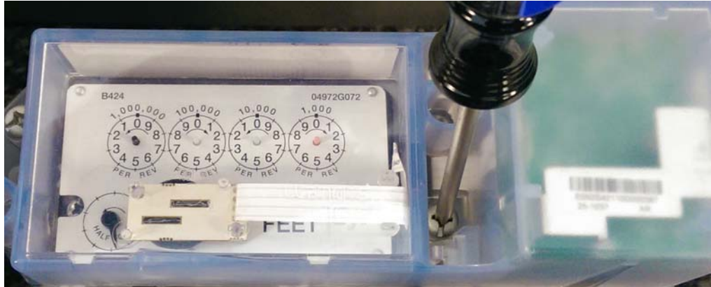
Figure 8 - 14. A Screw-holding Screwdriver Will Simplify Installing This Mounting Screw
