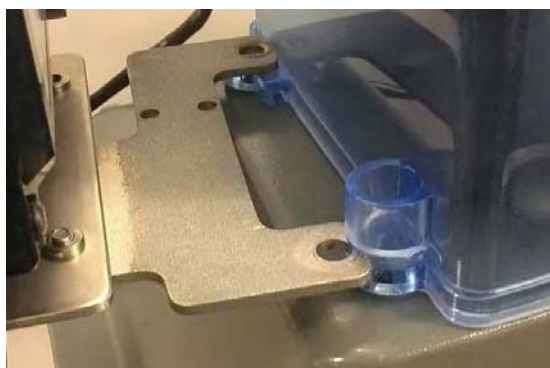
Figure 5 - 16. Slide Bracket into Index Cover Tamper Cup Slot
