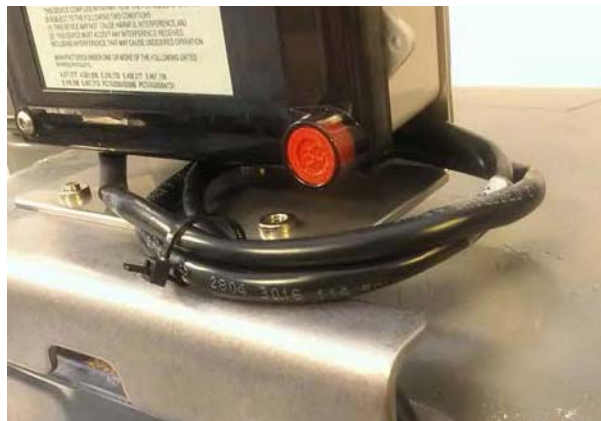
Figure 6 - 22. Cable Optionally Routed Above Index Cover Bracket
