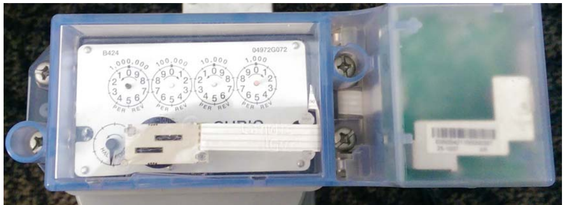
Figure 8 - 15. Index and Gridstream M120-1 Index Cover Installed
