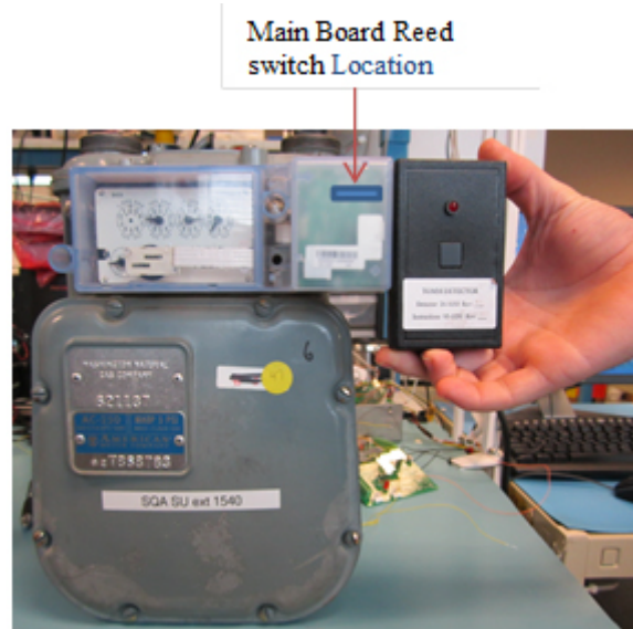
Figure 8 - 18. Main Board Reed Switch Location
