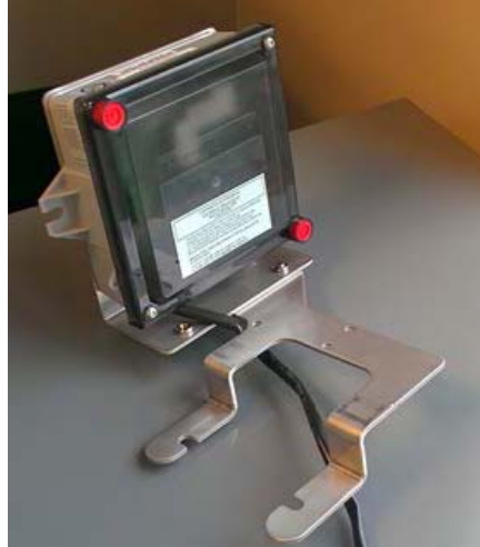
Figure 1 - 4. GPR with American Large Diaphragm brackets and hardware
