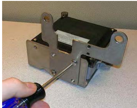
Figure 4 - 22. GPR Bracket Disassembly
