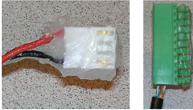
Figure A - 5. Apply the Compound to GPR Cable Connectors: Cover All Contacts
