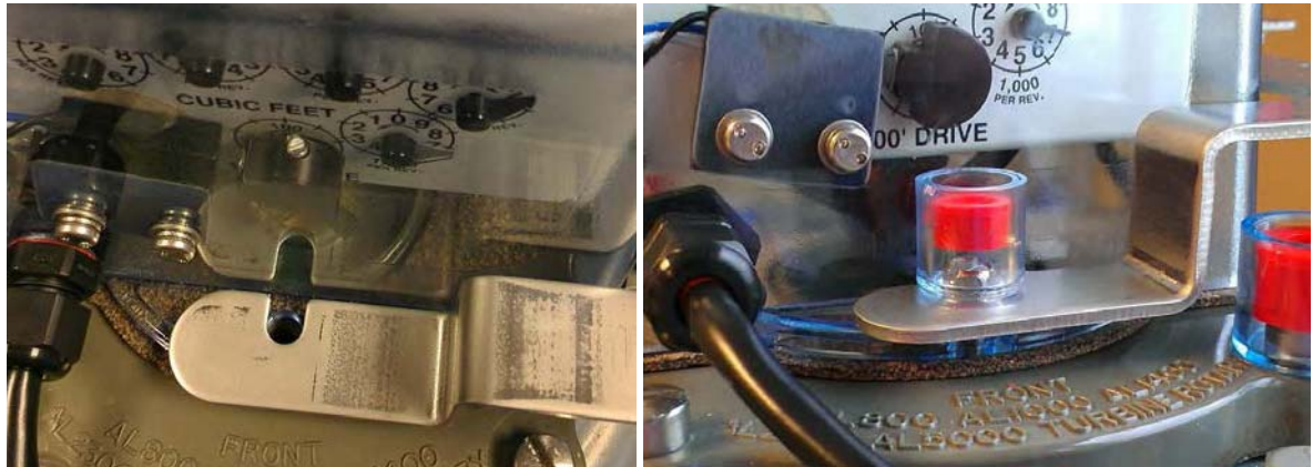
Figure 3 - 26. Tighten Front and Rear Cover Screws to 20 in-lbs ( \pm 5 in-lbs)
