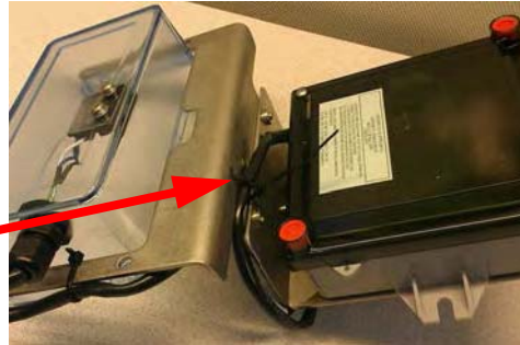
Figure 6 - 19. Excess Coiled Cable Attached Beneath GPR Bracket
