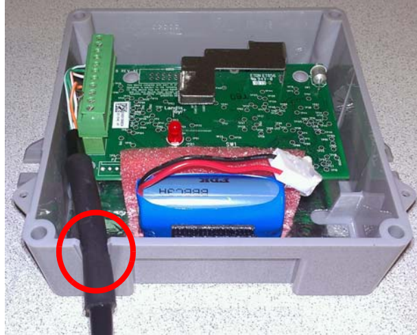
Figure 7 - 12. Pulse Interface Cable's Shrink Tubing Must Route Through GPR Strain Relief Slot
