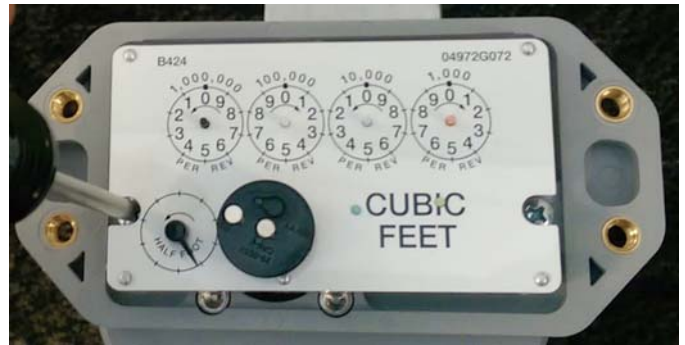
Figure 8 - 12. Attaching the Index
