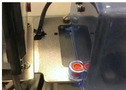
Figure 5 - 16. Slide Bracket into Index Cover Tamper Cup Slot
