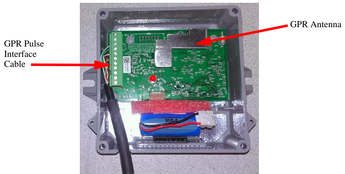
Figure A - 7. Arrange Cables As Shown Before Installing the GPR Cover
