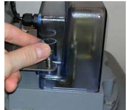
Figure 4 - 14. Install GPR Bracket, Screws and Tamper Cups
