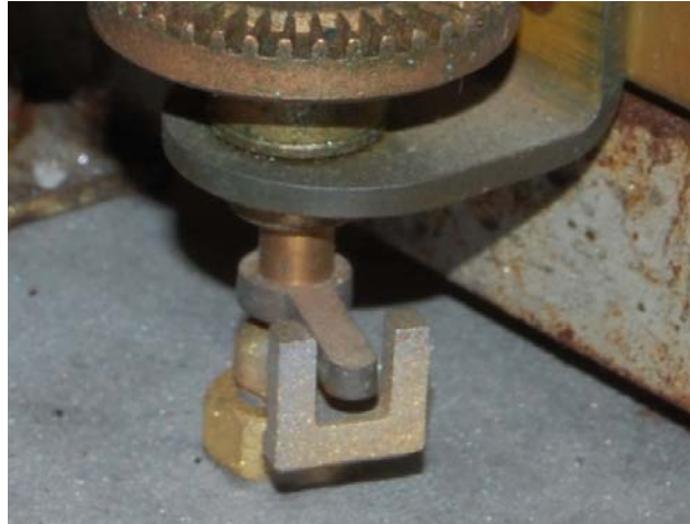
Figure 4 - 11. Index Drive Shaft Arm Alignment
