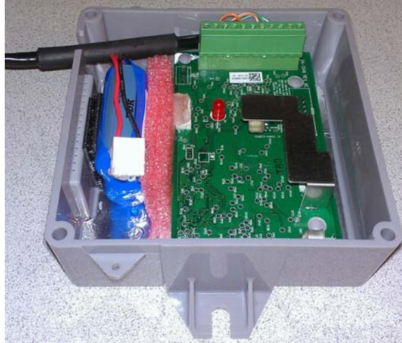
Figure 7 - 9. Cable to GPR Connection for a Single Form-A Volume Input
