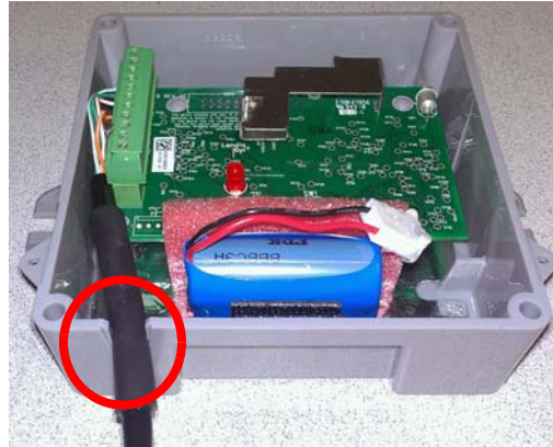
Figure 2 - 5. Pulse Interface Cable's Shrink Tubing Must Route Through GPR Strain Relief Slot
