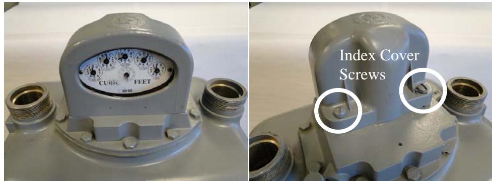
Figure 4 - 1. Rockwell Large Diaphragm Meter Index Cover Front And Rear Views
