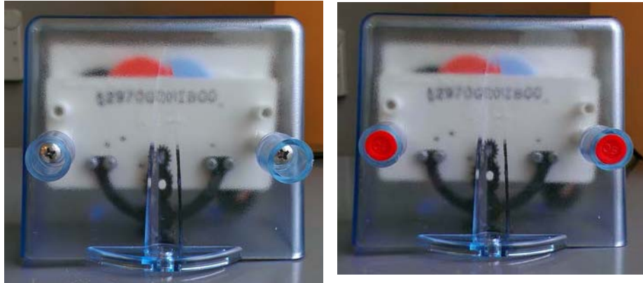
Figure 2 - 23. Install Index Screws and Tamper Seals
