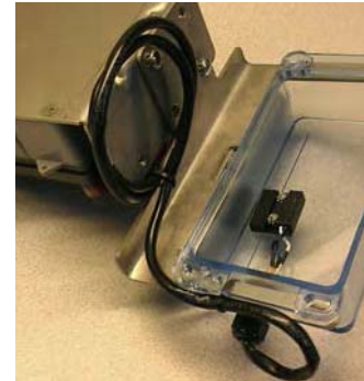
Figure 5 - 19. Excess Coiled Cable Attached Beneath GPR Bracket
