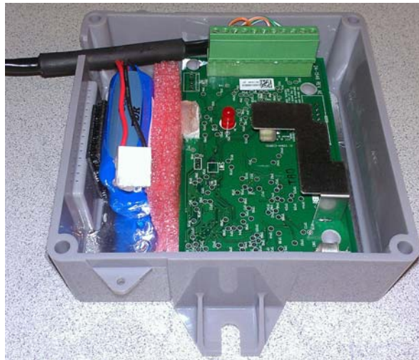
Figure 6 - 3. Cable to GPR Connection for a Single Form-C Volume Input
