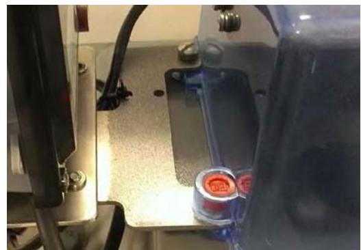
Figure 4 - 16. Slide Bracket into Index Cover Tamper Cup Slot
