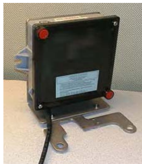
Figure 1 - 9. GPR with Rockwell Large Diaphragm Universal Hardware (kit 45-1186)
