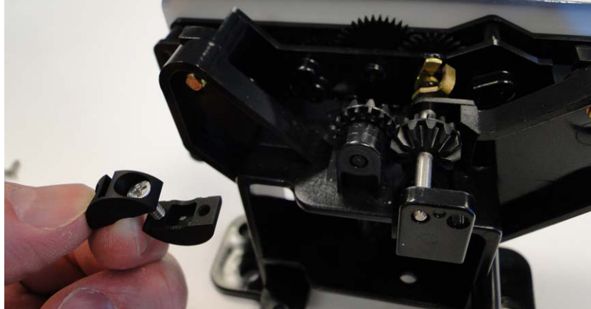
Figure 4 - 11. Slide Threaded Wheel Half Beneath the Index Drive Shaft
