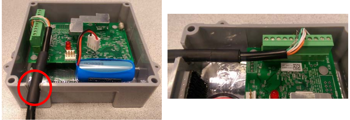
Figure 6 - 5. Pulse Interface Cable's Shrink Tubing Must Route Through GPR Strain Relief Slot
