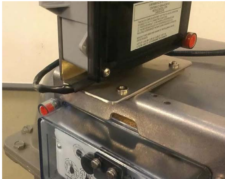
Figure 5 - 31. Do Not Route the Cable In Front of the GPR Bracket - Route the Cable As Shown in Figure 5 - 30
