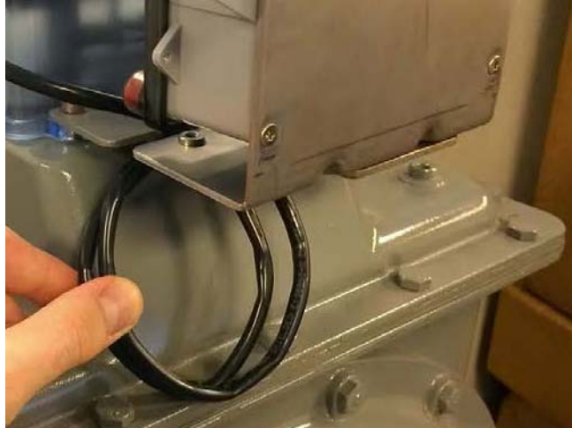
Figure 4 - 17. Coil the Excess Cable
