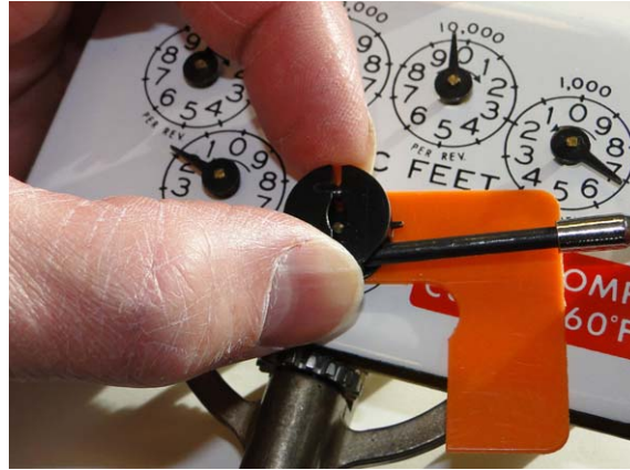
Figure 2 - 13. Insert 0.030 inch thick Shim and alternately tighten the Dial Wheel Screws to 3.5 inch-pounds ( \pm 0.50 inch-pounds).
