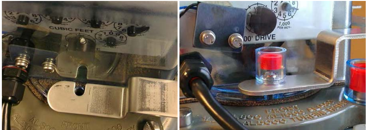
Figure 2 - 26. Tighten Front and Rear Cover Screws to 20 in-lbs ( \pm 5 in-lbs)
