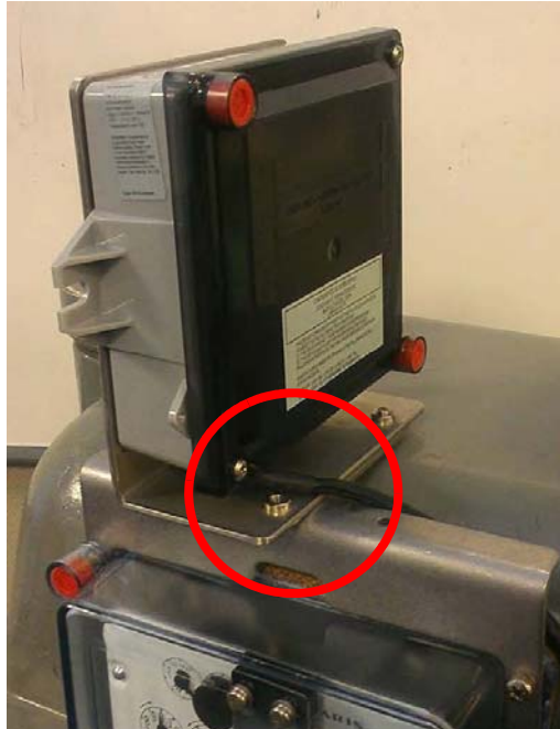
Figure 5 - 30. For Right-facing GPR Installs, Route Cable As Shown
