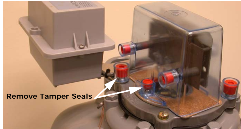
Figure 2 - 3. Remove Index Cover and Module Bracket Tamper Seals
