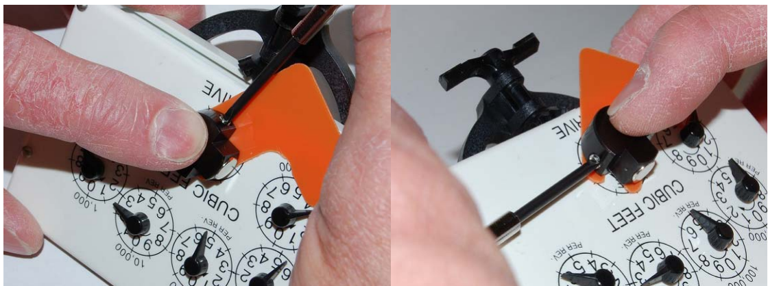
Figure 2 - 17. Tighten Dial Wheel Screws to 1.20 inch-pounds ( \pm 0.10 inch-pound)
