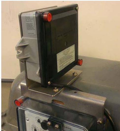
Figure 5 - 26. GPR Facing Right Side of Meter
