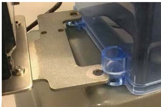
Figure 4 - 16. Slide Bracket into Index Cover Tamper Cup Slot
