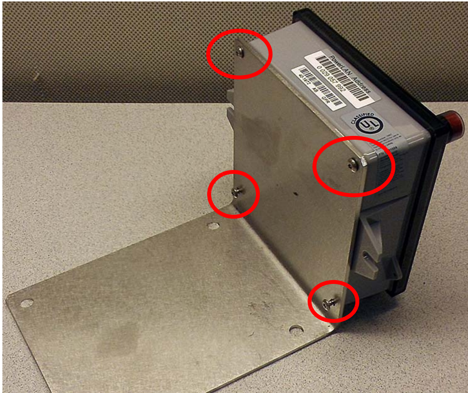
Figure 7 - 3. Attach GPR to Mounting Bracket
