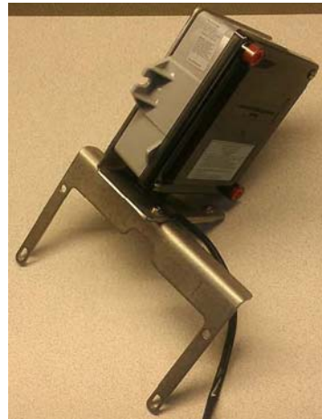
Figure 5 - 33. GPR Facing Right Side of Meter
