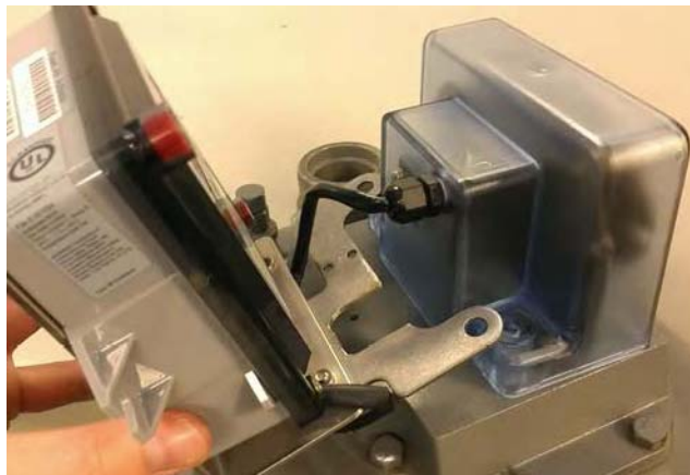
Figure 3 - 14. Install GPR Bracket, Screws and Tamper Cups
