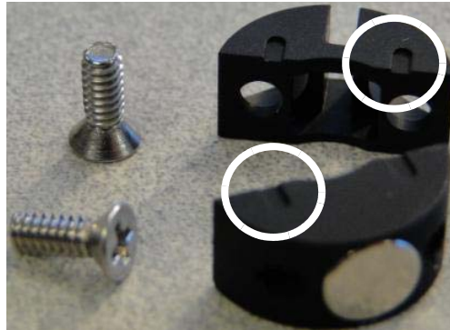
Figure 2 - 9. Where Alignment Slots Are Present On Index Face Mount Dial Wheels, The Slots Must Be Installed On Top
