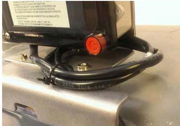
Figure 5 - 22. Cable Optionally Routed Above Index Cover Bracket
