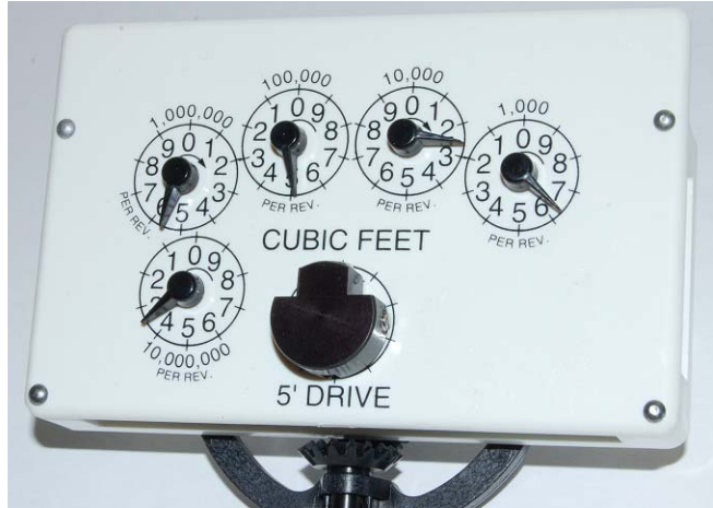
Figure 2 - 18. Balanced Dial Wheel Installed
