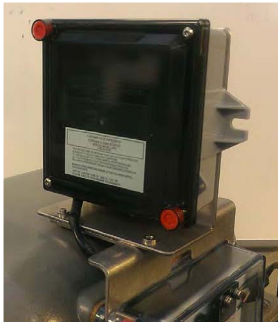
Figure 5 - 29. Left-Facing GPR Shown Extended Forward to Avoid Gas Pipe Interference
