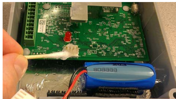
Figure A - 4. Force the Compound between Connector Pins
