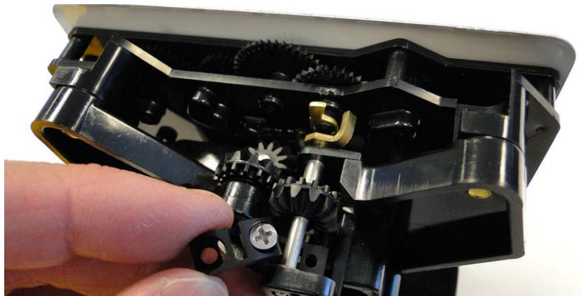
Figure 4 - 12. Slide Threaded Wheel Half Beneath Shaft
