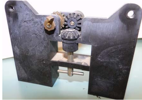
Figure 4 - 4. Index Removed from Unsupported Bracket Assembly
