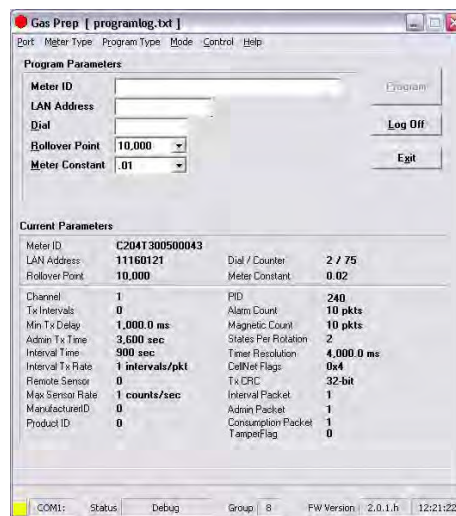
Figure 9.19 Re-Program Old With Module Plugged In
