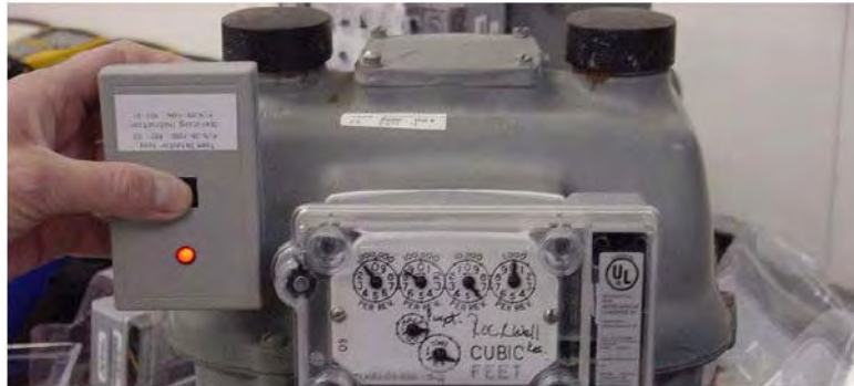
Figure C.2 Rockwell/Equimeter/Sensus RF Buster placement
