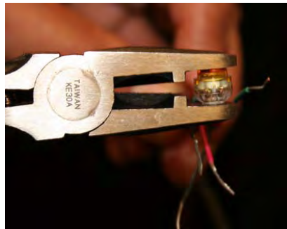
Figure F.2 ScotchLok Connector in Crimping Tool Jaws
