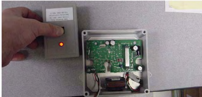
Figure C.6 ROOTS/Romets RG3 RF placement
