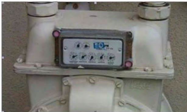
Figure 6.21 Sprague/Actaris: Indexes before installation
