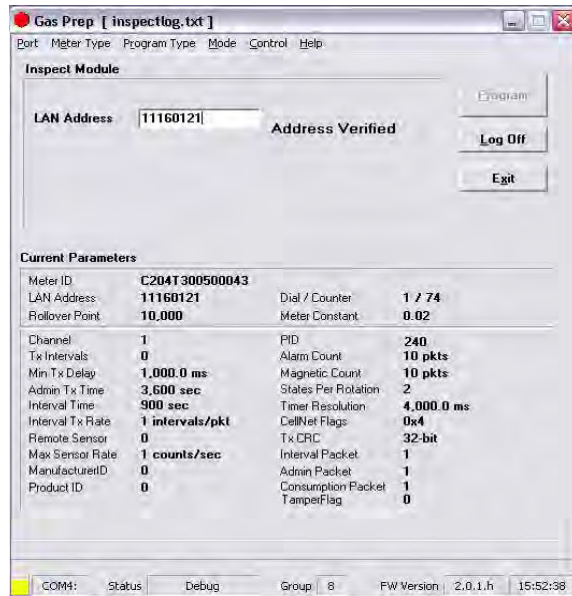
Figure 9.10 “Inspect Mode” With Power LAN Scanned In
