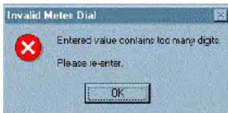
Figure 9.20 Error Message Displayed when Entered Read is too large for the Rollover Point
