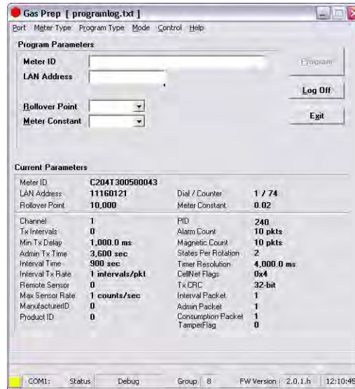
Figure 9.12 “Program New” Screen with Module Plugged In
