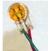
Figure F.1 Wires Pushed into Scotchlok Connector
