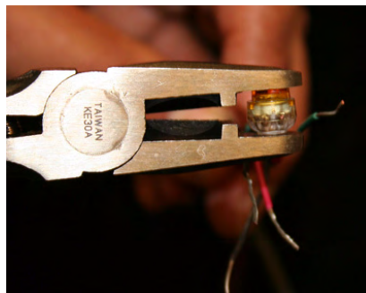
Figure F.2 ScotchLok Connector in Crimping Tool Jaws
