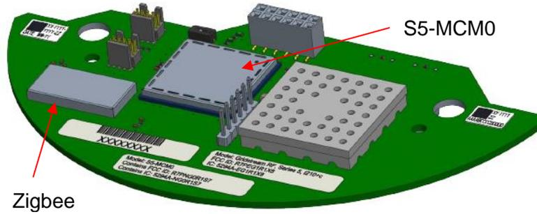
**Figure 2. I210+c module, top side with shield lids installed**
