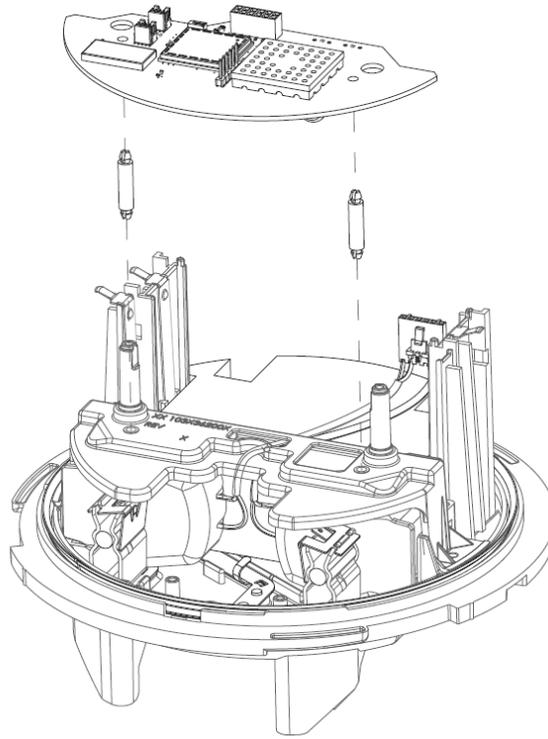
**Figure 5. I210+c module installation view**
