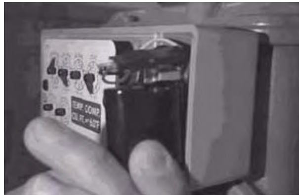
Figure 5.10 American: Installing the battery with the battery cable on top
