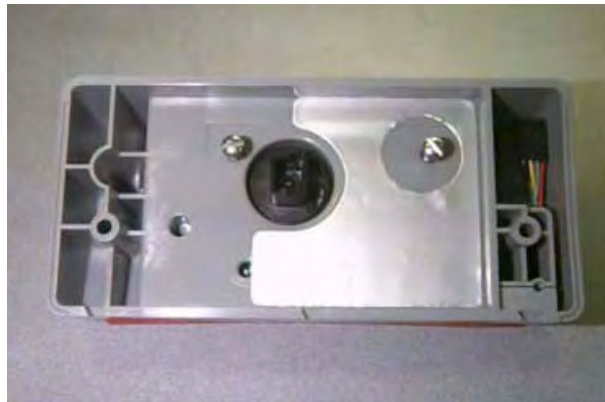
Figure 5.46 Lancaster/National: Meter Module pre-assembled
