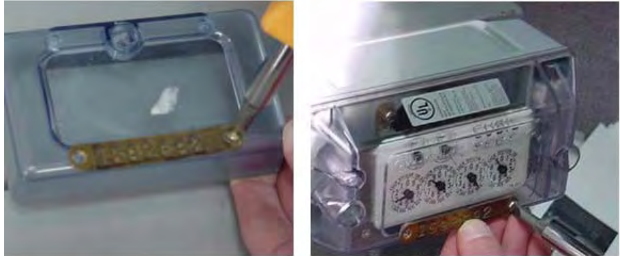
Figure 5.53 Lancaster/National: Replacing Serial Number Plate
