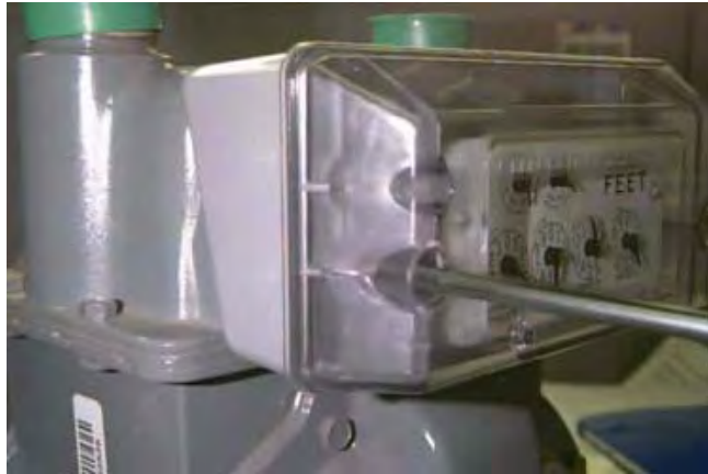
Figure 5.37 Sprague/Schlumberger/Actaris: Fasten Cover Screws and Insert Tamper seals
