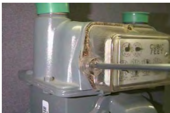
Figure 5.27 Sprague/Schlumberger/Actaris: Removing the index cover
