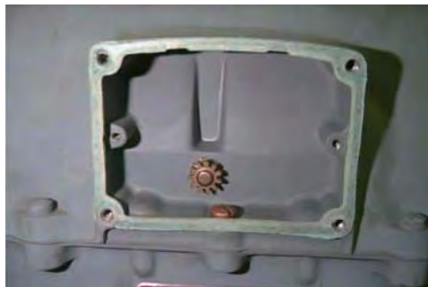
Figure 5.15 Rockwell/Equimeter/Sensus: Meter with tamper seals and index cover removed
