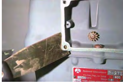
Figure 5.16 Rockwell/Equimeter/Sensus: Removal of index cover gasket
