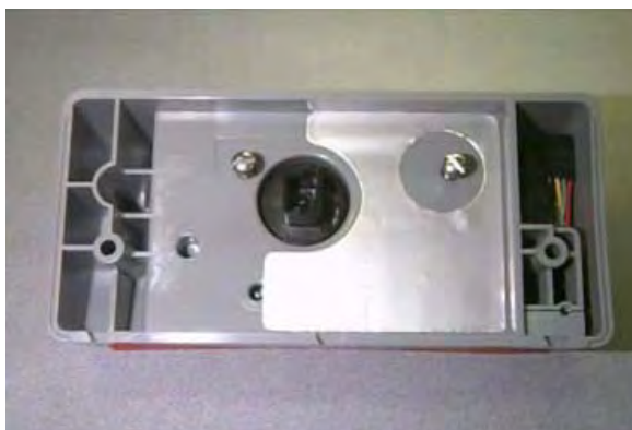
Figure 5.25 Sprague/Schlumberger/Actaris: Meter Module before installation
