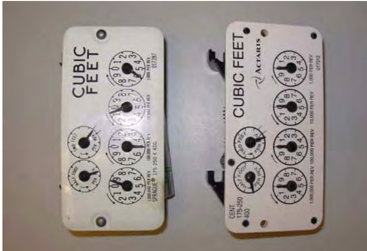
Figure B.2 Metal rivets on a Sprague cover
