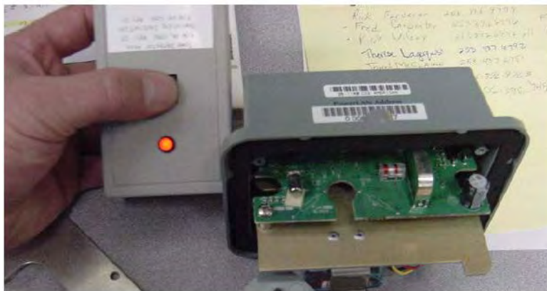
Figure C.5 Commercial Gas Module uncovered
