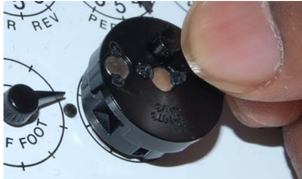
Figure 5 - 11. Installing the Dial Wheel Pin
