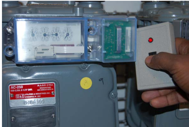
Figure 5 - 15. RF Buster oriented to Meter Module for testing
