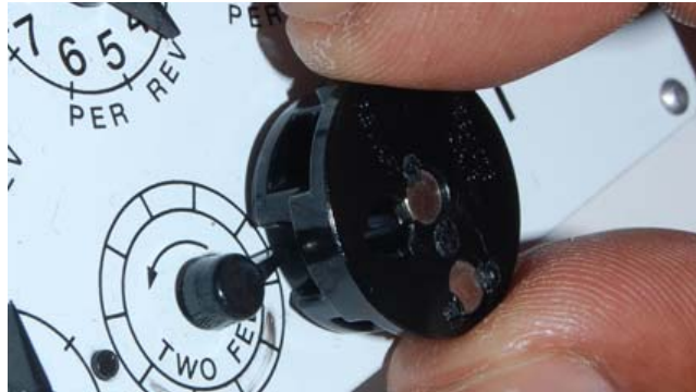
Figure 5 - 8. Dial Wheel with pointer slot positioned for pointer entrance
