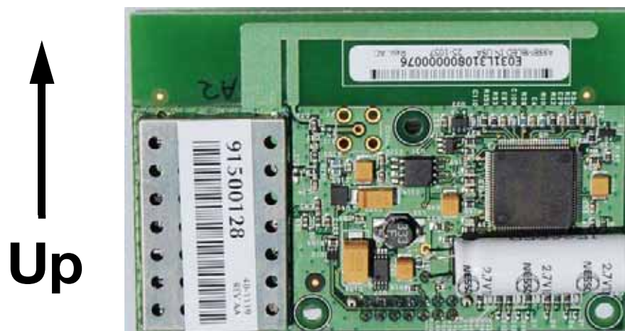
Figure B - 1. Recommended Board Orientation for Optimal Antenna Performance
