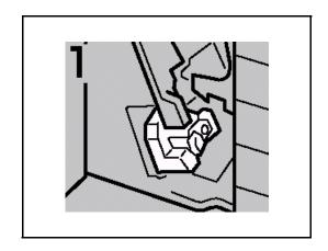
2 Hold the green lever and pull out the cartridge gently.
