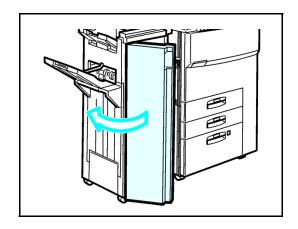
Pull out the Punch-out container and properly dispose of the punch-outs.
