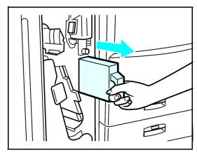
3 Slide the Punch-out Container back into the Finisher and close the Front Cover.
