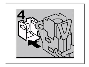
6 Align the arrows on the new refill and the cartridge, and then push in the refill until it clicks.
