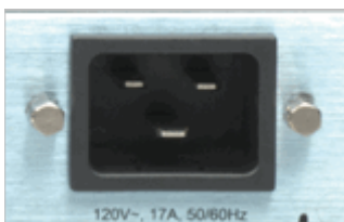
Figure 4-2. AC Power Input
