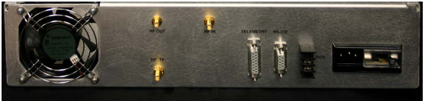
Figure 7 Rear Panel Showing Interlock Terminal Board
