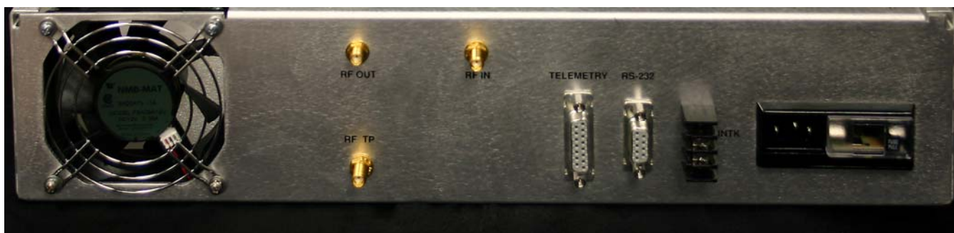
Figure 7 Rear Panel Showing Interlock Terminal Board
