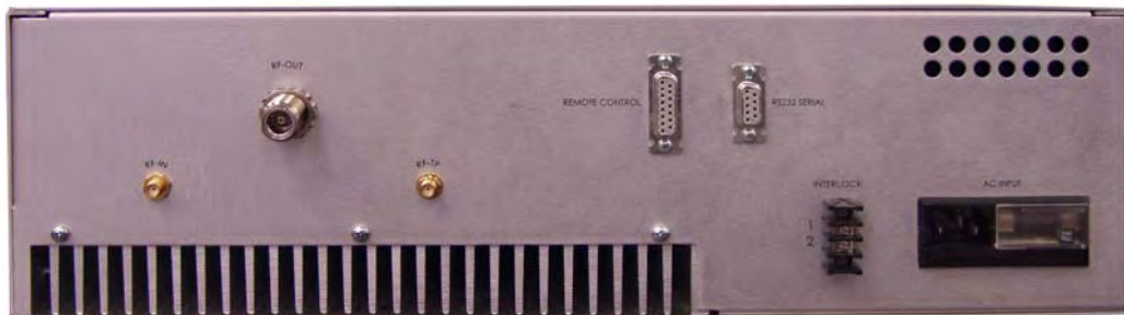
Figure 7 Rear Panel Showing Interlock Terminal Board
