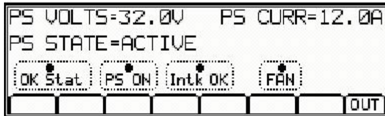
Figure 6 Power Supply (P/S) Submenu Screen
