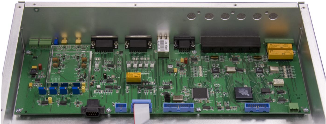
Figure 15 CPU Board Shown Mounted in the Control Chassis
