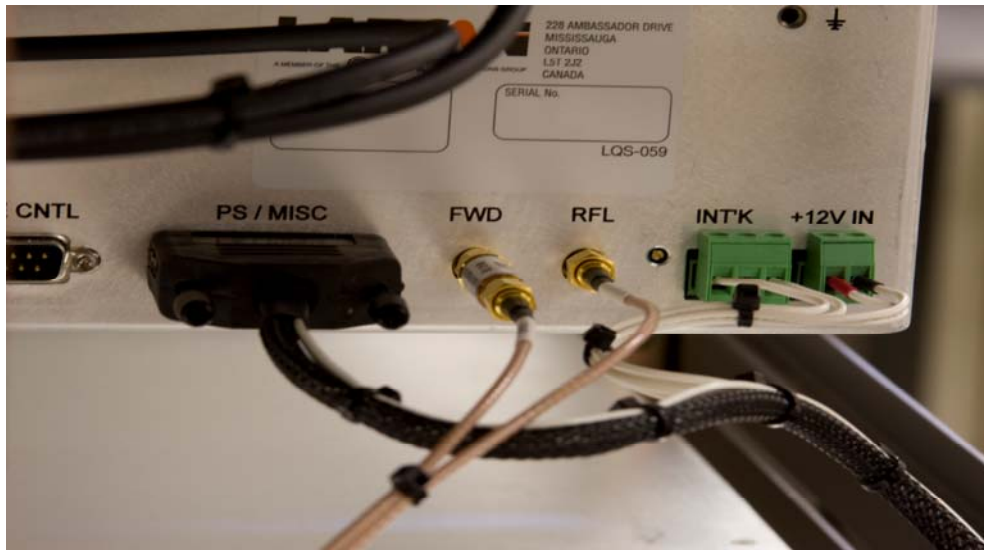
Figure 5 Rear Panel Showing Interlock Connector
