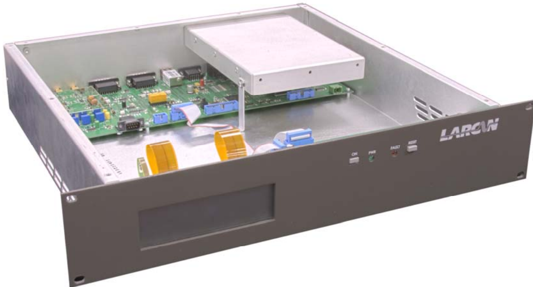
Figure 4 Main Transmitter Controller
