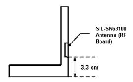
c) For minimum distance less than 3.9cm, the orientation of the RF chip shall be restricted to place the A1 marker located at the top.
