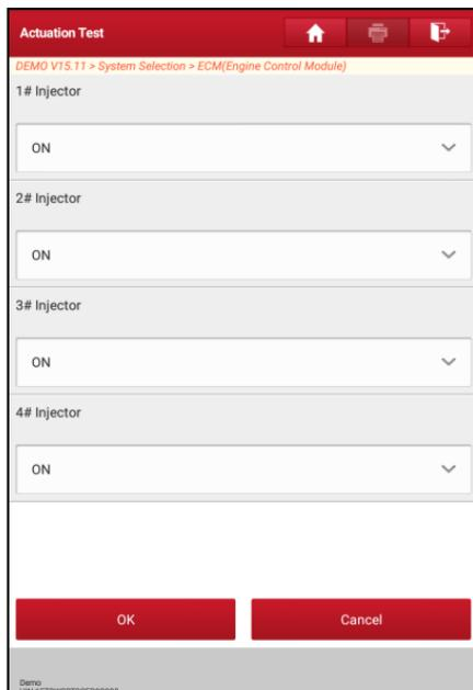
Simply follow the on-screen instructions and make appropriate selections to complete the test. Each time when an operation is successfully executed, “Completed” displays.
