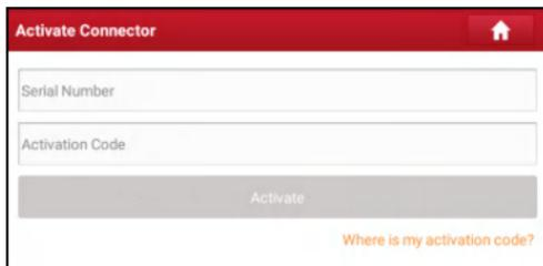
Input the Serial Number and Activation Code, and then tap **Activate** to activate the VCI.
