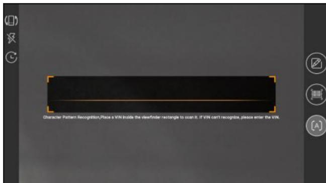
Place the VIN inside the viewfinder rectangle to scan it. The most recognizable location for this number is in the top left corner on the vehicle's dashboard. Other locations include the driver's door or post, and the firewall under the hood.
