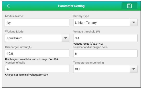
In addition, due to the pack terminal of EVB624 does not participate in the discharge test process in discharge equalization mode, number of cells does not need to be set.
