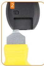
Use the tool into the gap to separate the shell
