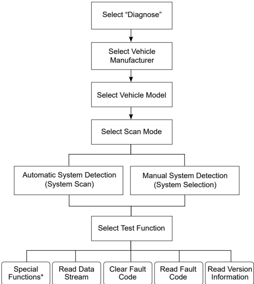
Take DEMO V15.34 as an example to demonstrate how to diagnose a vehicle.
