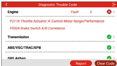
In above figure, the tested system with fault code is tagged with a red cross and the system with OK displays with a green tick.
