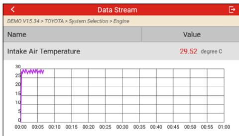
Combine: Tap it, a pull-down list of the data stream items appears on the screen. Select the necessary items (Max. 4 items can be selected at the same time) and the screen will display the waveforms corresponding to these items immediately.
