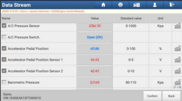
DEMO V14.95 > Demo > System Selection > ECM(Engine Control Module)
