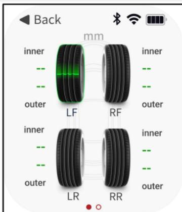
3. The system starts the detection from the left front wheel of the vehicle by default, but you can also manually select any tire for detection. After clicking on the tire icon, attach the magnetic head of the device to the tread of the corresponding tire, and press the measurement button on the device to start the detection. At this time, a scanning animation is displayed on the
