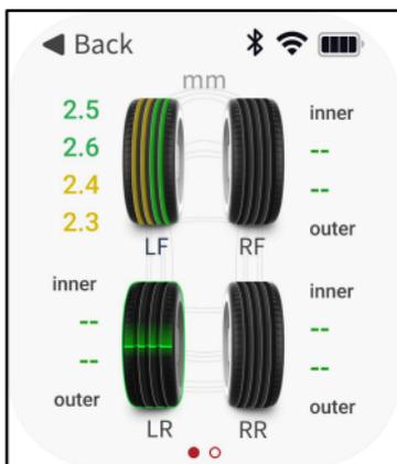
5. After all tire tests are completed in turn, the tire icon will identify the tire detection results in different colors.
