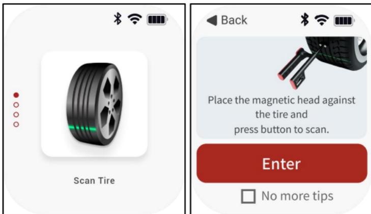
2. Read the detection method prompted on the screen and click **Enter** to go to the tire tread detection interface.
