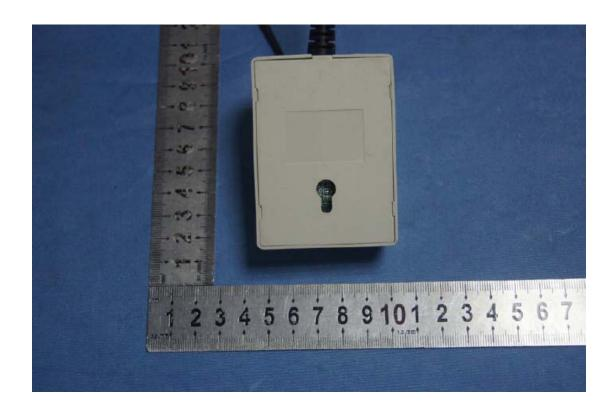
The system power supply is provided by the USB of PC. The power supply is 5.0V. The computer communicate with RF by the serial port DB9.
