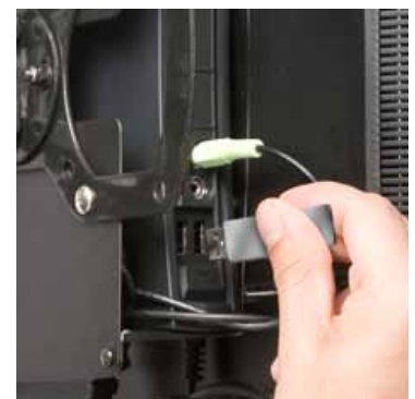
Insert a USB drive into the Qtrac to immediately start playing new media.
