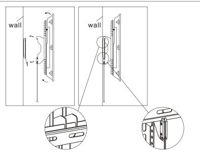
(1)Press the brackets after you put them on the wall plate, then they would be locked with wall plate.
