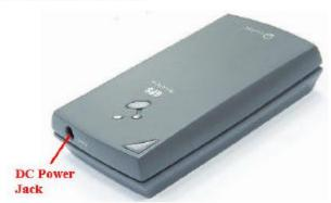
The Bluetooth GPS has two LED light which each has two colors. One is GPS & Charge status LED, that is named LED 2, and the other is Bluetooth & low power status LED, that is named LED 1. The status table of LED shows as follows:
