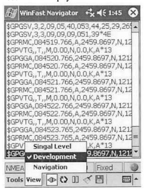
\*PS: After using the navigator software, please remember to disconnect (click "Tool" -> Disconnect) or exit to release the COM PORT so it can be used by other navigation software.
