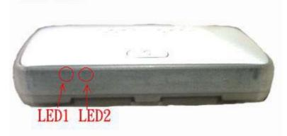
The Bluetooth GPS has two LED light which each has two colors. One is GPS & Charge status LED, that is named LED 2, and the other is Bluetooth & low power status LED, that is named LED 1. The status table of LED shows as follows:
