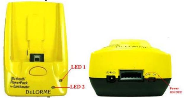
The PowerPack for Earthmate GPS with Bluetooth has two LED light which each has two colors. One is GPS & Charge status LED, that is named LED 2, and the other is Bluetooth & low power status LED, that is named LED 1. The status table of LED shows as follows:
