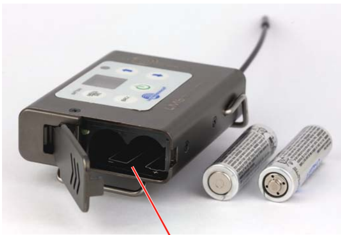
Battery polarity is marked inside the compartment
