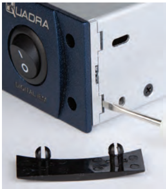
Plastic guards snap out from corners. Pry out the aluminum inserts on the side panel with a small screwdriver.
