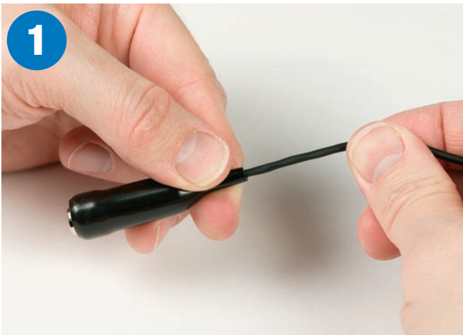
1 Pull the sleeve over the connector so the ends of the connector and sleeve are almost flush.
