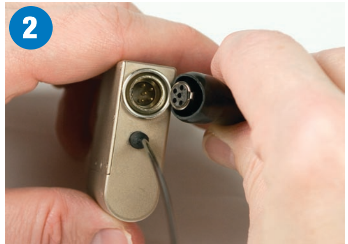
2 Align the pins on the plug and jack and insert the connector.
