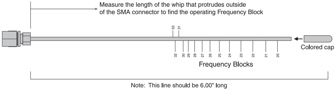
All Lectrosonic UHF transmitter antennas follow the color code specifications in the chart below to identify operating frequency block range. (The frequency block range is engraved on the outside housing for each individual transmitter.)
