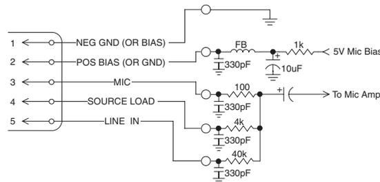
The best RF protection is accomplished by installing RF bypass capacitors at the mic capsule. If this is not possible, or if you are still having problems, capacitors can be installed on the mic pins inside the TA5F connector housing.
