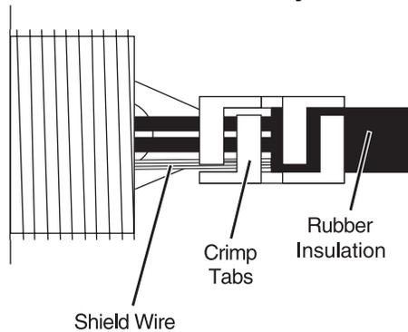
**NOTE:** This termination is required on VHF transmitters and will still work fine on UHF transmitters.
