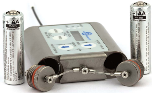
AA battery compartments are O-ring sealed
