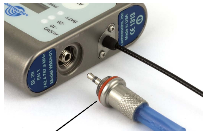
Treat O-ring with petroleum jelly before connecting (see below)
