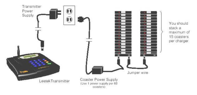
\*Smps adaptor (Transmitter Use: DC 12V 2.5A) , (Charger Base: DC12V 2.5A)
