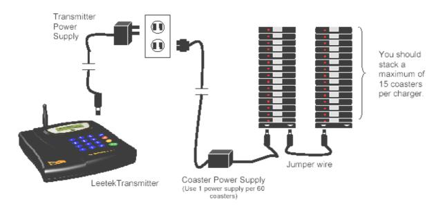
\*Smps adaptor (Transmitter Use: DC 12V 2.5A), (Charger Base: DC12V 2.5A)
